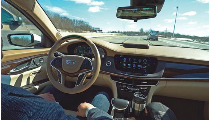
2. Cadillac's Super Cruise, offered on its 2018 CT6 sedan, permits hands-off driving but warns the driver if he/she diverts attention. (Source: Cadillac)
