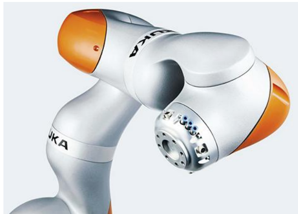
3. KUKA's LBR-iiwa industrial robot uses machine learning for increased safety for human/robot collaboration. (Courtesy of KUKA)
