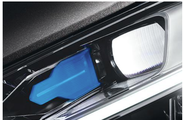
3. The European version of the Audi laser light doubles the range of the high beam. (Source: Audi)
