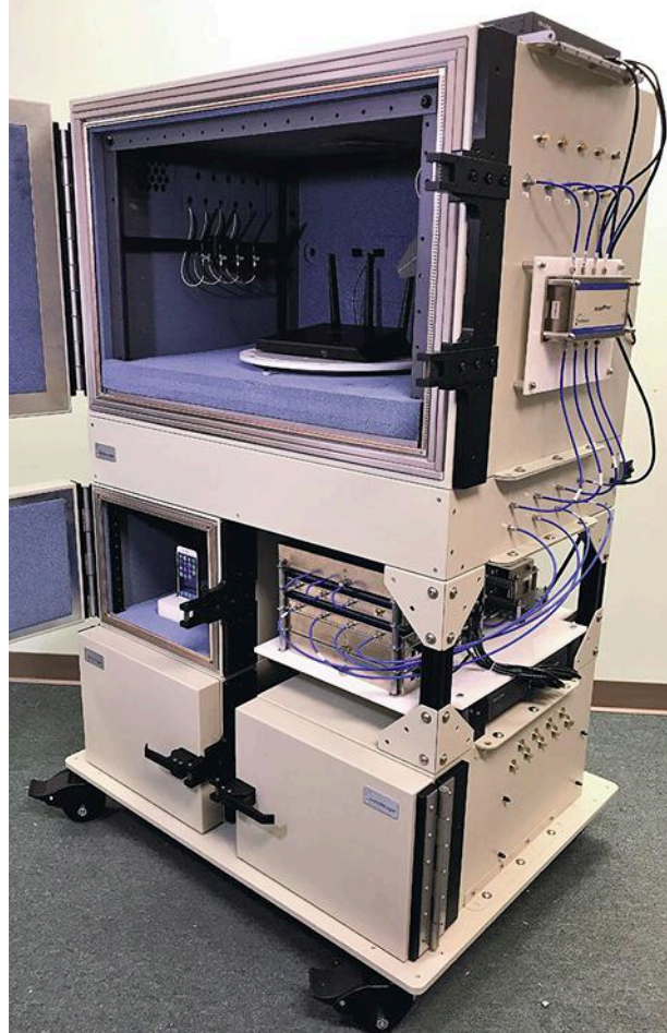
3. The octoBox personal wireless testbed allows fully OTA testing and coupling between AP and STA, at any location. (Courtesy of octoScope)
