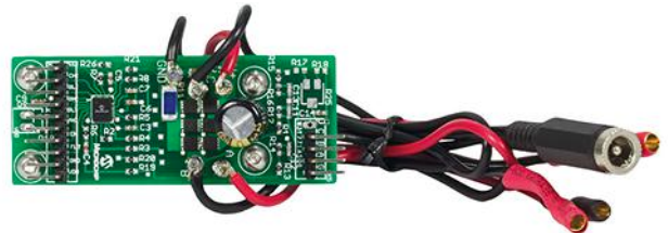
Microchip's MIC4607 is an 85-V, three-phase MOSFET driver with adaptive dead-time, anti-shoot-through, and overcurrent protection.
