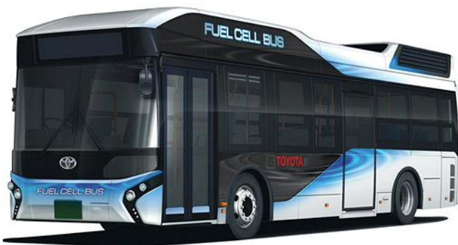
4. Toyota's Sora bus has 10 tanks containing 600 liters of hydrogen.
